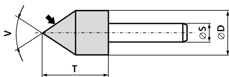
Mounted point, cylindrical with conical end 5211 - D \times T \times S - V
